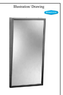
**Frame** — 18-8 S, type 304, heavy-gauge stainless steel with satin finish. Tapers from 4" (100mm) depth at top to 1" (25mm) depth at bottom. Bevel design on front holds frame tightly against mirror. Corners are welded, ground, and polished smooth. Galvanized steel back and inner stiffener frame is one-piece welded construction with slots for mounting screws and integral screw-head lock.
